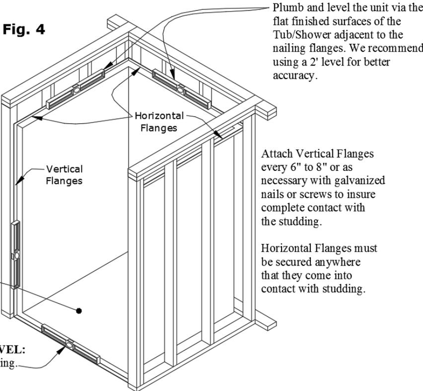
After securing the floor flange re-check that proper slope has been achieved in the shower floor. Assure that there are no dips, humps, or other restrictions in the shower floor which will prevent proper water drainage.
